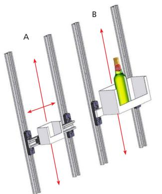
A - ASCENSORE A 2 ASSI A - 2-AXES ELEVATOR
